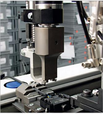
The application was accomplished with 35 kHz components and differential weld path limitation systems integrated into a special-purpose system.
