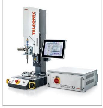
The application was produced on a torsional TSP750 SONIQTWIST<sup>®</sup> welding system with MAG generator and TCS5 controller, or with corresponding components in a special system.
