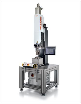
The application was produced on a USP8000 welding machine with a two-stage anvil unit.
