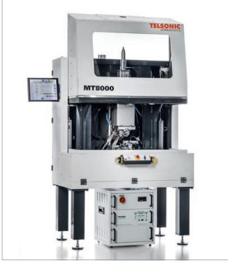
The application was created using a 10 kW MT8000 PowerWheel® system, retractable sound protector and TCS5 welding process control.
