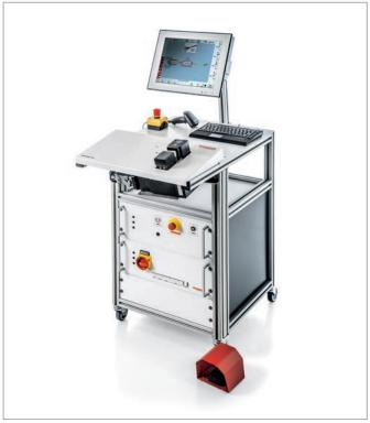
The application was created using a 3.6 kW TS3 TTelso®Splice wire splicing system with attachments suited to working with aluminium.
