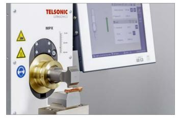
The application was produced on a 20 kHz MPX ultrasonic welding system and Telso<sup>®</sup>Flex control software, as well as with corresponding components integrated into a special system.
