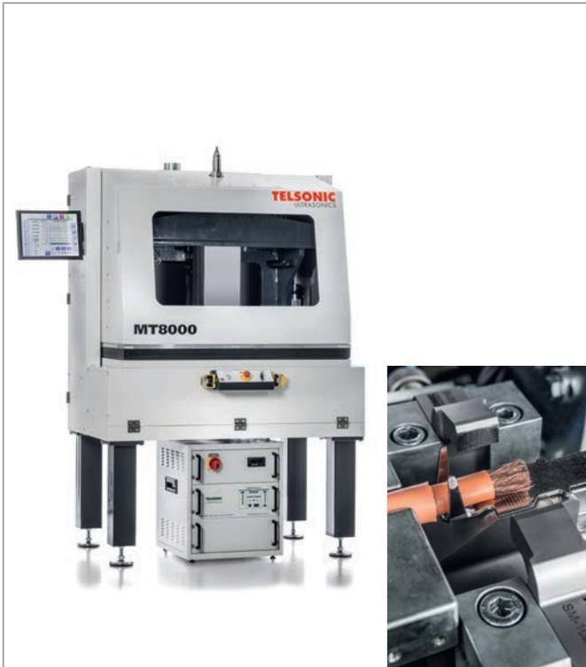
The application was created using a 10 kW MT8000 PowerWheel® system and TCS5 welding process controller with touchscreen operation.
