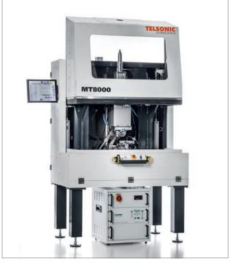
The application was welded using a 10 kW MT8000 PowerWheel® system and TCS5 welding process controller.
