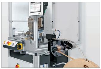
The application was produced on a linear 20 kHz MPX ultrasonic welding system and suitable special equipment.
