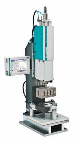
The application has been produced using a USP8000 welding system / the appropriate components in a bespoke system.
