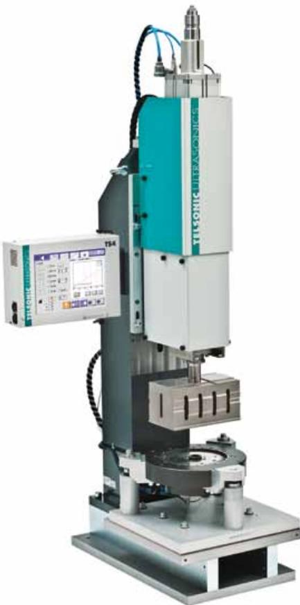
The application has been produced using a USP8000 welding system with appropriate 2-stage process tools.
