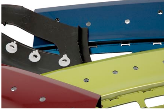
Image no. 27-01 TC_Soniqtwist_4Teile.jpg The torsional ultrasonic welding procedure of Telsonic AG delivers best results in joining plastic parts, such as distance sensors, cable clips or fixing pins, to painted exterior parts in automobile manufacturing.
