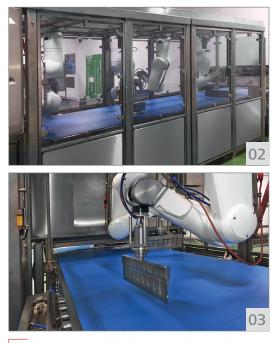
01 The new 760mm blade from Telsonic further enhances02 the efficiency and productivity from robot mounted03 ultrasonic systems used on tray bake products.
