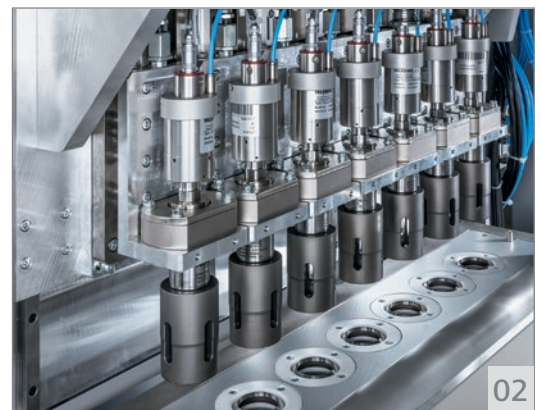
01 Coffee pods with filter felt 02 Ultrasonic cutting and welding systems
