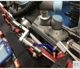
O1 Mounting ultrasonic welding technology to a robot, or as shown here, a Cobot provides a highly flexible solution
