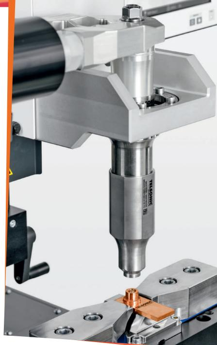
**1.** Ultrasonic welding pole - The application requires welding to take place at the bottom of the cylindrical cell through the jelly roll, so the ultrasonic welding tool has to have a long reach.
