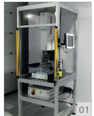
01 Telsonic programmable, servo driven indexing machine for pleated lip welding. The machine HMI also displays multiple weld recipes
