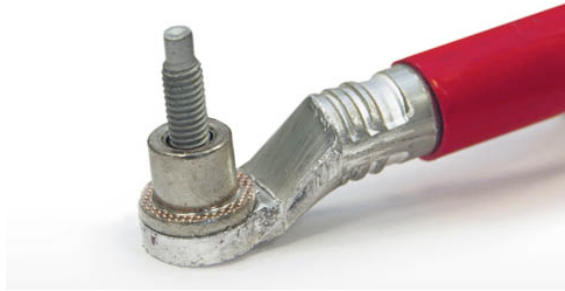
Image No. 36-01 TC_LO-Anschlussbolzen.jpg Designed for the supply of electricity in Jaguar cars: interface stud welded to a LEONI aluminium busbar using TELSONIC's torsional ultrasonic welding technology.
