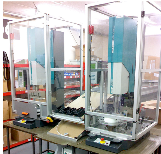
(Telsonic Ultrasonic Systems – Welding both Socket Sub-Assemblies and Modules for CMD)
