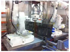
robustness and design of the converter for mounting to the robot, the exceptional cut quality and low noise operation. Telsonic's scope of supply included 20kHz 500mm long single length blades, Telsonic MAG-WO20024-S generators and the aseptic SE2024-4/IP67 converter, designed for food cutting applications with integral cooling ports.
