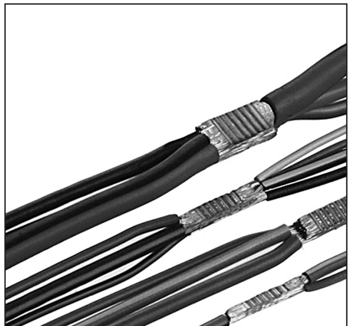
Typical Copper Wire Splices
