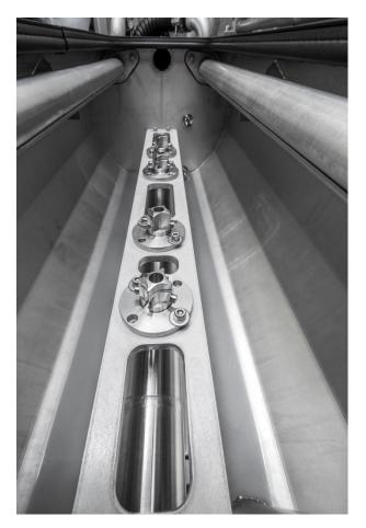
The ultrasonic chambers have a special design which optimizes the use of the ultrasonic radiation from the two tube resonators. The cleaning chambers shown here are each fitted with an ultrasonic tube resonator from Telsonic. Telsonic supplies tube resonators of the type RS-25-55-P in various lengths and can produce power of up to 1200 W with a suitable generator. The tube resonators boast a compact design, a 360-degree ultrasonic vibration field and efficiency of over 95%.
