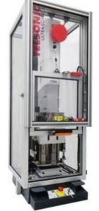
Telsonic's solution for this application is based upon dual USP2000 20kHz 3kW presses, each of which uses titanium multi-tip tooling. The product nests comprise of poured resin cavities which are also spring loaded to protect the product "A" surfaces and ensure good collapse control on the delicate staking tabs. All of the tooling is interchangeable across both machines to support flexibility in production and also provide high levels of future-proofing for next generation variants.
